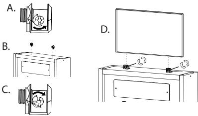
Attach double side tape to the back of the mirror as shown. Attach mirrors (x2) to side panels. Begin by starting screws #6 x 1/2"(x2). Do not tighten! Slide mirror to side and remove tape on back of mirror. Align mirror so it is vertically straight. Press on to rail and finish tightening screws. Do not over tighten screws!!
