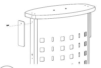
Attach case holder to the display top using #6x 5/8" assembly screws
