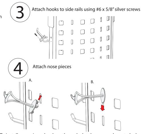
To Install nose piece, hook up through slot then press down to lock as shown above
