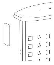
Attach case holder to the display top using (2) #6 x 5/8" screws
