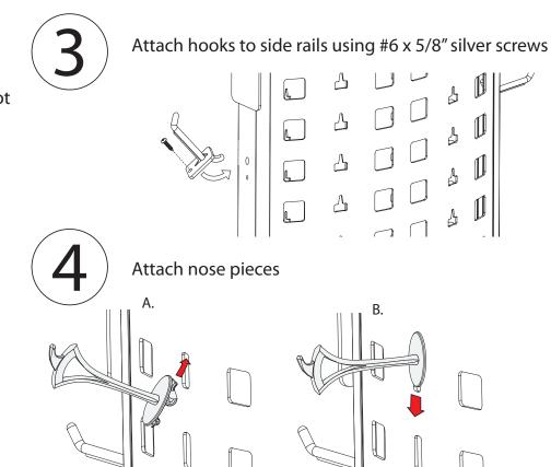
To Install nose piece, hook up through slot then press down to lock as shown above
