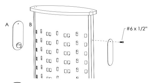
Locate the #6 x 1/2" (x2) screw from box 1. insert the accessory hook then screw in.
